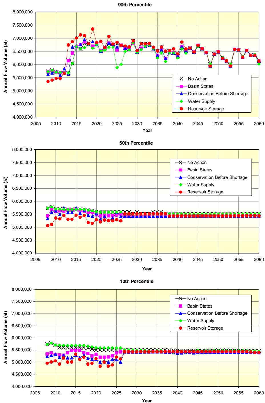
Figure 4.3-36 Colorado River Annual Flow Downstream of Palo Verde Diversion Dam - RM 133.8 (af) Comparison of Action Alternatives to No Action Alternative 90 th , 50 th , and 10 th Percentile Values
