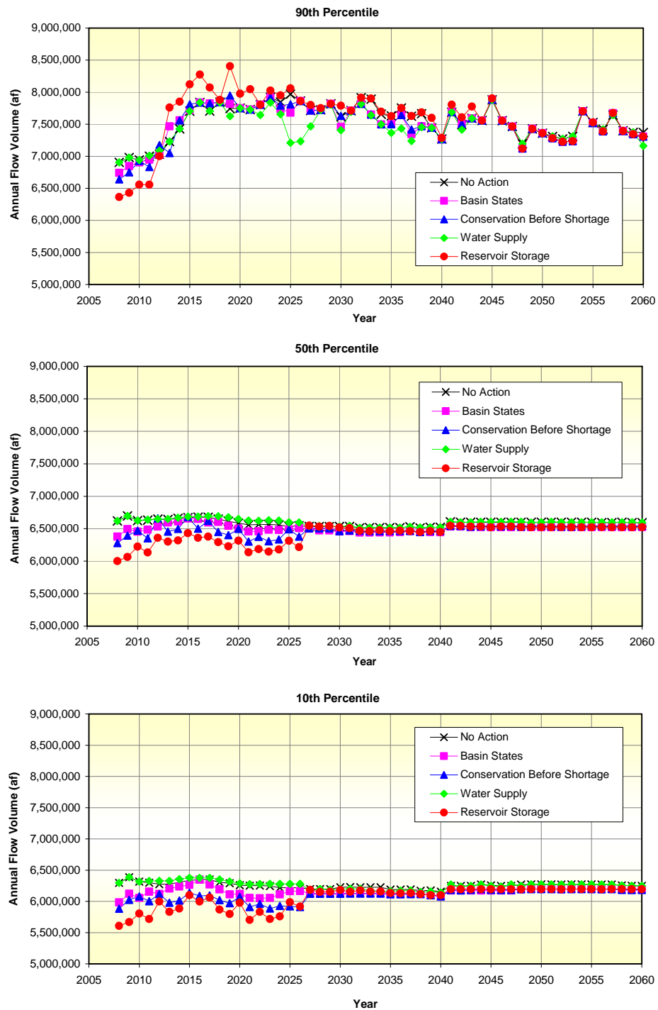
Figure 4.3-35 Colorado River Annual Flow Upstream of CRIR Diversion - RM 180.8 (af) Comparison of Action Alternatives to No Action Alternative 90 th , 50 th , and 10 th Percentile Values
